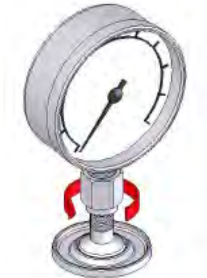
Figure 2-2. Connect Assembly to Test Port
