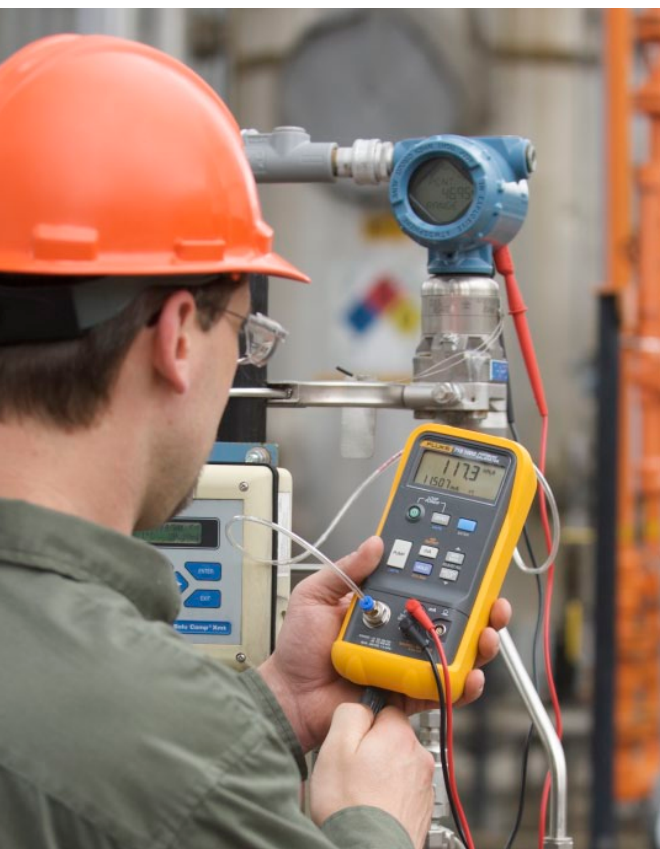
Fluke 719 Electric Pressure Calibrator
