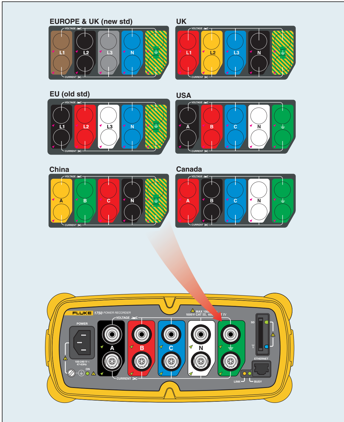
Figure 2. Applying the Front Panel Decal
