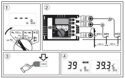
Figure 4. R<sub>A</sub> 3-pole Measurement
