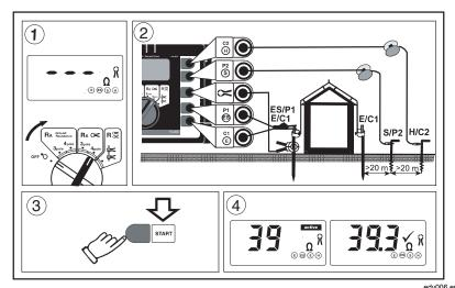
Figure 7. R<sub>A</sub> 4-pole Selective Earth Resistance Measurement with Current
