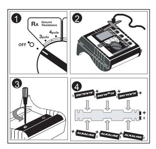
Figure 2. Inserting Batteries
