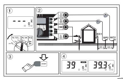
Figure 6. R<sub>A</sub> 3-pole Selective Earth Resistance Measurement with Current Clamp
