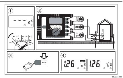
Figure 8. Stakeless Ground Loop Measurement
