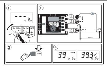
Figure 3. R<sub>A</sub> 2-pole Measurement
