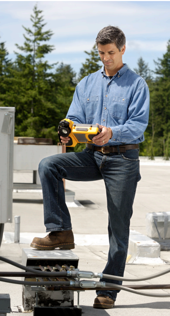
Performing a routine roof inspection to search for moisture (leaks and wet areas) in the roofing materials. Note: These tests are typically done at night, this photo is for marketing purposes only.
