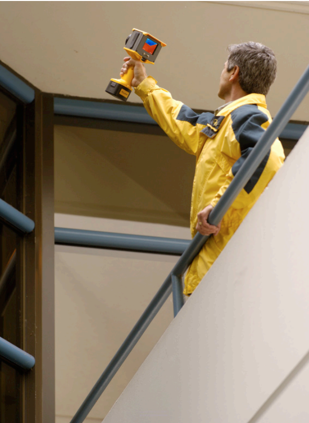
Checking for moisture within the wall surface with a Fluke InSight Thermal Imager.
