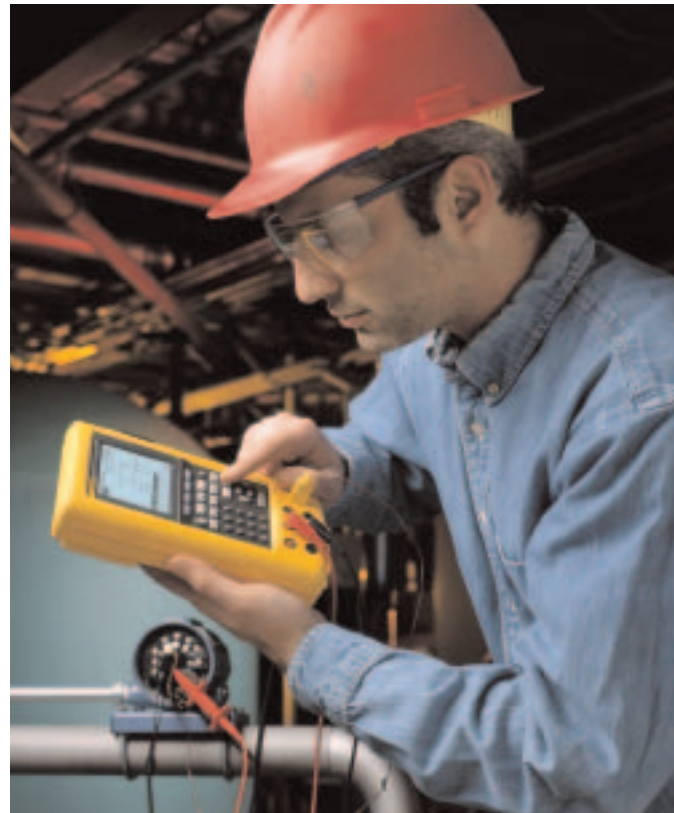
The Fluke 744 HART documenting process calibrator allows technicians to calibrate, maintain, and document HART-based field devices without the need for additional equipment.
