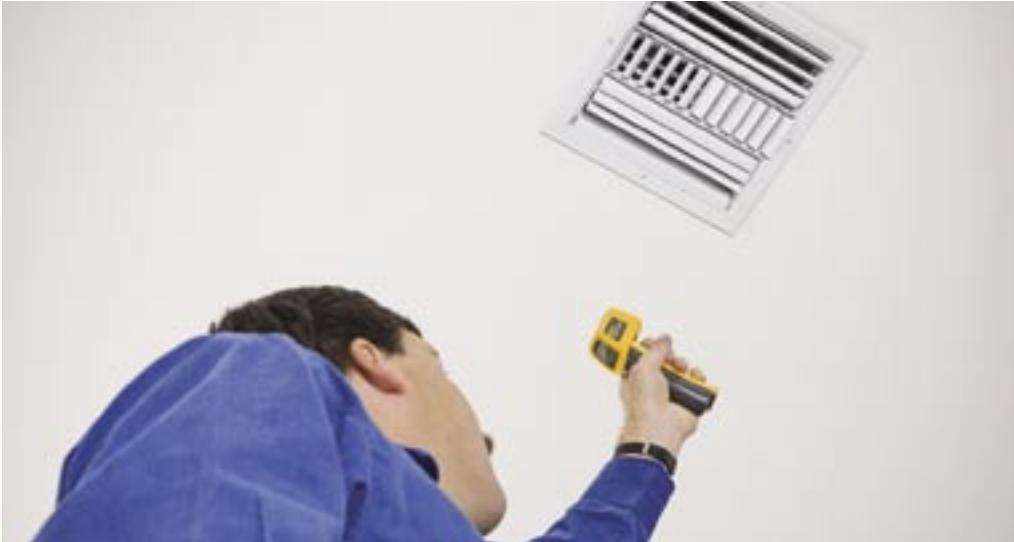
Use non-contact temperature measurements for inaccessible targets.
