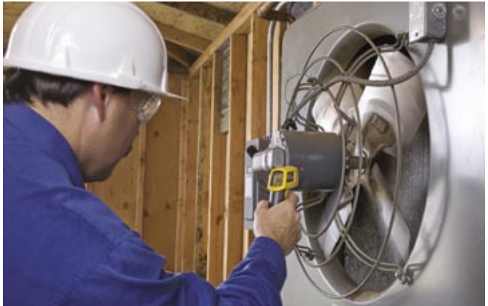
Check motor temperatures quickly, without contact.
