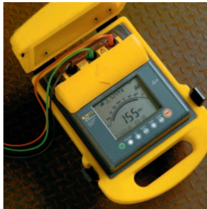
PG&E technicians used the Fluke 1550 to check for insulation degradation as an integral part of their intensive preventive/predictive maintenance program.
